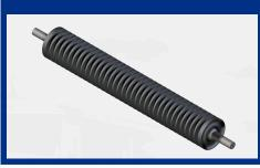
Live Shaft Idlers are provided with pillow block bearings. They are typically used in feeder applications or applications with higher belt tensions not suitable for conventional flat rollers with internal bearings. Live Shaft Idlers are available in impact, spaced rubber disc and steel configurations.
